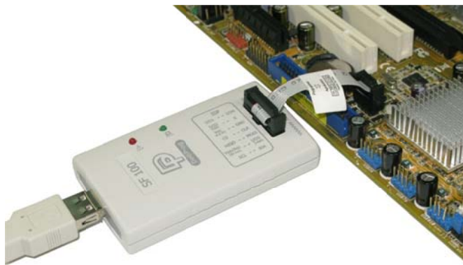
Fig 2: SF100 connected to the application pin header
