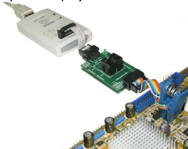
Fig 3: Backup Boot Flash (BBF) connected to SF100
